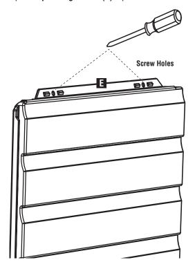
Snap Repeat Right Side (E) into the back position of Repeat Floor (B).
